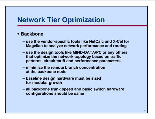
Vendor-provided tools are specifically designed for their switches and therefore would improve the topology designs created by generic tools like Mind-Data. Generic tools design networks based on tariffs, generic routing and preset delay requirements. These designs must be fine tuned with the vendor-specific tools. For example Nortel's NetCalc is an excellent tool for analyzing various topologies to find the optimum solution for the backbone.
