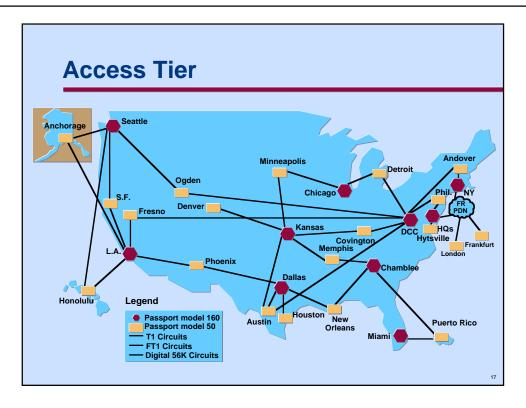
This design provides one hop access connectivity to the backbone. Hence the total hop count for any access location to any access location through the backbone is 4 hops or less. The number of hops depends on the performance requirements for each application.
