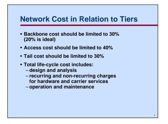
Allocating cost to each tier of the network makes the network design easier. Each tier can be designed independently once the backbone locations are identified. The life-cycle network cost is divided into three pots: Backbone, Access and Tail.
