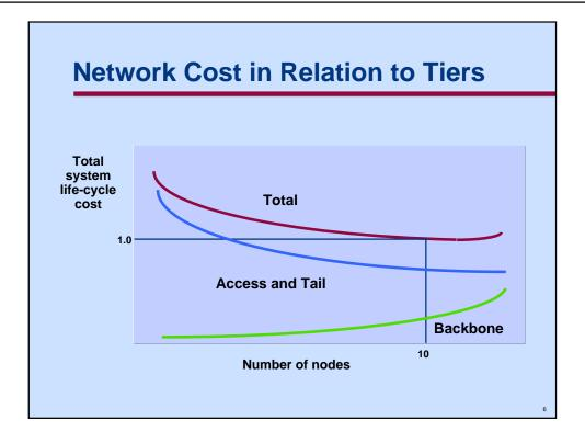
This chart shows the normalized total network cost versus the number of backbone nodes. The life cycle cost decreases as the number of backbone nodes increase up to a certain number. This number is 10 nodes in our case study.
