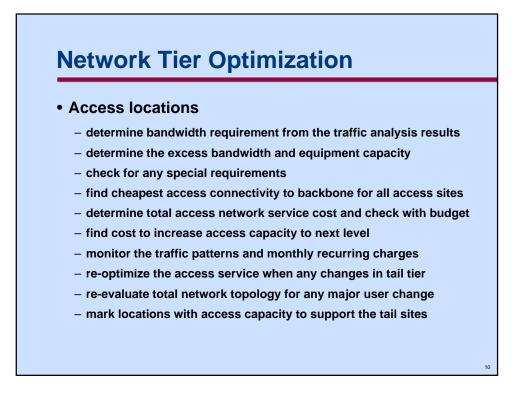
Bandwidth requirement is calculated by (traffic volume)x1/(ckt utilization factor): i.e. 23000 bit/s \* 1/(0.5) = 46000 bit/s ~ 56K or 64K circuit and it has access capacity for 5-9 kbit/s data.
