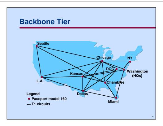
Each regional office has a PBX that is connected to the host PBX via T1 bandwidth in the existing network. Our design uses a 2:1 compression in the backbone for each voice channel when the bandwidth is needed, otherwise it is not compressed.
