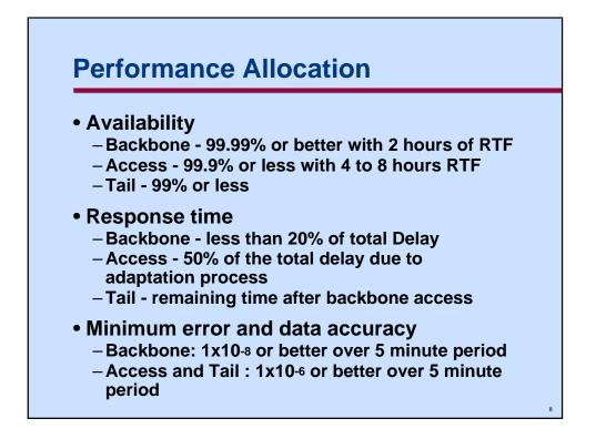
The backbone network is the most stringent tier with the highest reliability and the shortest response time to failures (99.99% or better with 2 hours of RTF) so that transport service outages are minimized.
