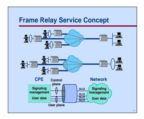
Frame relay is built around the principle of multiplexing logical connections over a single physical facility. The connection is controlled by several components which also double as the basis for the tariff definition offered by the provider.
