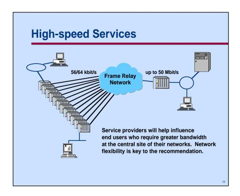
Most customers have deployed frame relay in a star topology, similar to their previous leased line network. In this configuration, one location functions as the central point of traffic for one to many remote locations. The central point of the star typically requires the most bandwidth because more traffic passes through it than any one of the remote locations.
