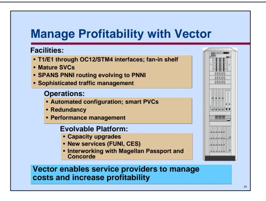
Nortel's Magellan Vector is designed to enable service providers to manage costs. The highest priority was placed on Vector providing a substantial level of redundancy. Redundant power supplies and fans were provided on Vector from the outset, with an imminent release (available in August of this year) providing redundant processors and switch fabrics. Electrical port redundancy will be available in early 1997, with optical port redundancy soon thereafter.
