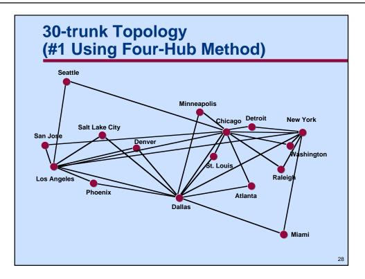
This is one of the two four-hub topologies done as part of the exercise. The hubs are Chicago, New York, Dallas and Los Angeles, which are directly connected to each other. The other cities are connected to the nearest two hubs, with one exception (San Jose).
