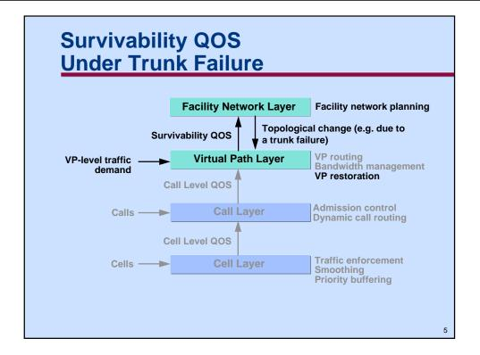
The survivability functions of the network, which are among the most difficult aspects of network design, VP routing design, bandwidth management capability, and fast VP restoration design are all in the upper two layers. The concept of survivability quality of service (SQOS) is introduced in [2].
