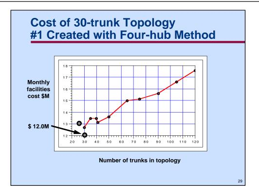
As has happened several times before in Nortel's design experience, a simple four-hub design prepared in a few minutes has seemingly come out of nowhere to win the contest. At the least, this is an approach one should use to keep other designs honest, because it can be done so easily.
