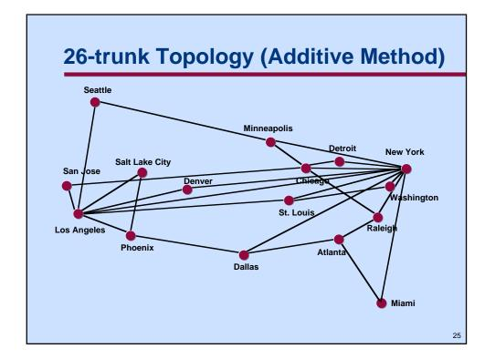
This shows the 26-trunk topology designed using the additive approach.
