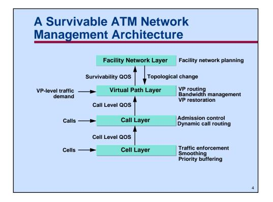
Two of the reference papers, [1] and [2], explain the network management layering concept, and the diagram above from [2] is a useful summary. The purpose of the layering is to simplify the network management process, which, in its broad sense, includes everything on the chart above.
