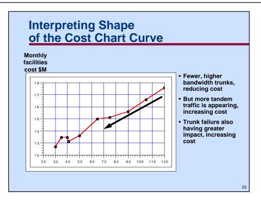
The three effects in the note on the right of the slide are important. Fewer trunks are better in terms of lower cost per kbit/s. But fewer trunks means more tandem traffic. And a more massive impact due to failure, which must be covered (but not for OC-12 in this particular case study). So often, depending on reliability requirements, the traffic profile, and tariffs, the curve bottoms out at some point and then starts to go back up as the number of trunks is further reduced.
