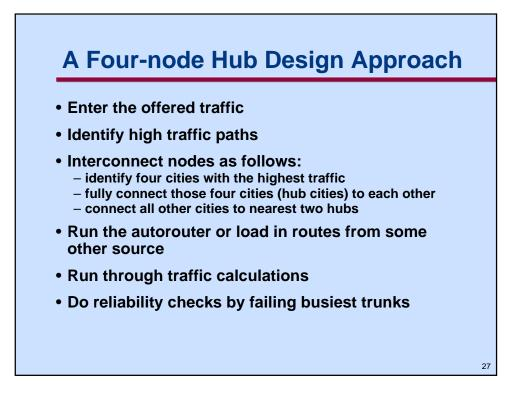
Several variations of the multi-hub design approach have worked well in network designs at Nortel. One can start with two hubs, and home all other nodes to those two nodes. Or one could use three hubs, or four or five, and connect other nodes to the nearest two hub nodes. As the number of hubs increases, tandem traffic increases on hub-to-hub connections. Often four hubs are the most cost-effective. With the hub approach, the hubs themselves are usually fully meshed.
