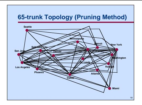
This is not an optimum topology in an age where high-bandwidth fiber is much cheaper than T3 on a per-kbit/s-basis. For the design above, there is actually a lot of fiber, but not enough yet. (Due to the low resolution of the picture, there was no attempt to identify fiber on it).
