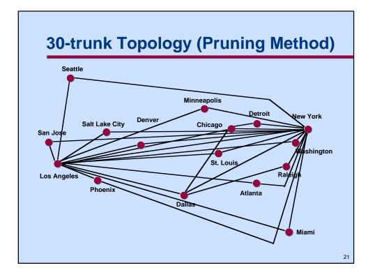
Here, failure scenarios must be done quite rigorously, because many nodes only have the minimum allowable two trunks. If one fails, only half the traffic carrying capacity remains, so those two connections must be tested for adequate bandwidth.
