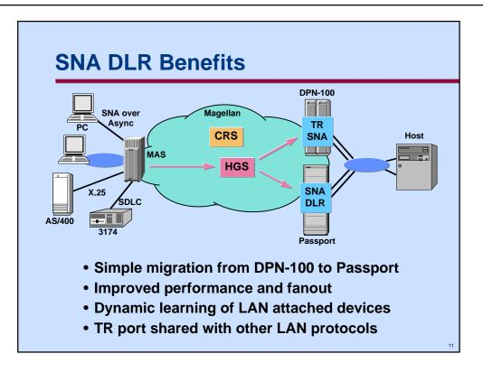
Migration from the DPN-100 token ring SNA service (TR SNA) is straightforward as the Passport service offers a superset of the DPN-100 capabilities. Using the HGS or CRS, the migration from DPN-100 to Passport can be done without changes to the installed base of DPN-100 equipment or remote devices. It also allows redeployment of displaced DPN-100 equipment.
