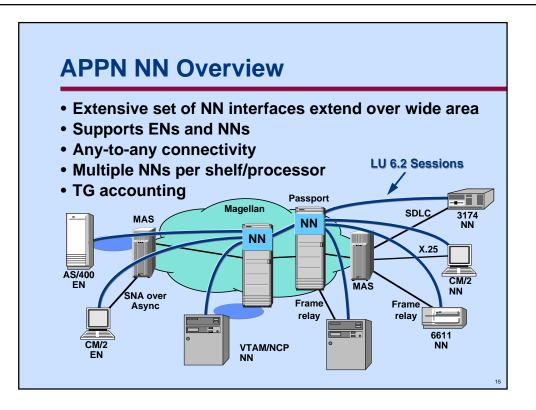
The Magellan implementation is much more than a simple box solution. A major difference of the Magellan implementation over other vendors' implementations is the extension of the interfaces over the wide area network (WAN). Allowing the interfaces to extend over the WAN allows the network operator to take full advantage of Magellan networking features and to protect the existing DPN-100 investment.
