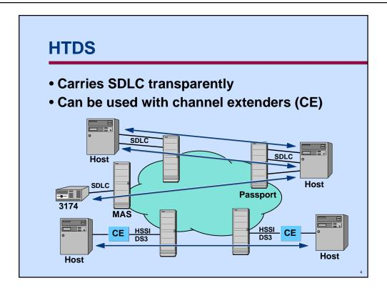
The HTDS service simply carries SDLC frames end to end. For each link coming into the network, there must be one link at the other end of the network. Idle flags are suppressed to optimize use of network bandwidth. Since no local termination is performed, multi-link transmission groups continue to be supported for legacy SNA.
