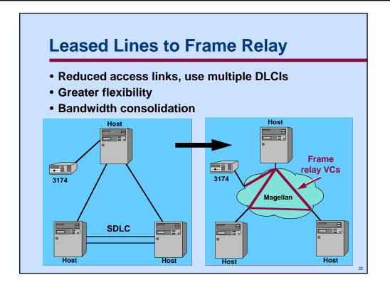
Migrating from SDLC leased lines to frame relay is relatively simple. Typically, hardware upgrades are not required. Reconfiguring an SDLC line to frame relay is trivial.
