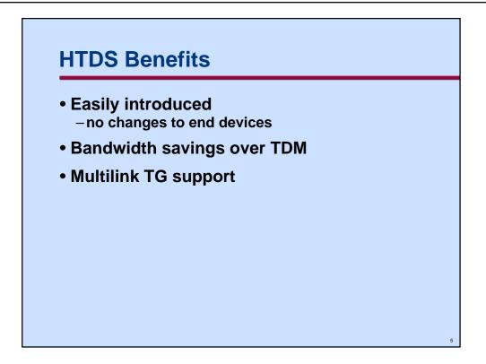
HTDS is simple to introduce. End devices continue to use SDLC or channel extenders and the frames are simply transported across the network to another SDLC attached device or channel extender.
