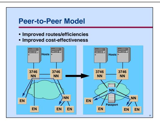
In the above example, sessions between ENs in the network must traverse back to the data center. By introducing the Passport NN in the network, communications between the ENs can be done more efficiently by avoiding having to go through the data center.
