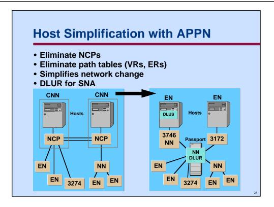
The NCP in a network is not a standalone APPN node. It must always be combined with VTAM to form a composite network node (CNN). With APPN, the NCP can be eliminated (along with its software licence) by replacing it with a 3746 NN (or alternatively a 3172). Without the NCP, VTAM can then become a simple EN.
