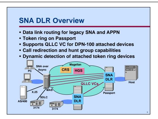
SNA data link routing (DLR) is the evolution of SNA on DPN-100. It provides functionality that is very similar to the existing DPN-100 token ring SNA service. It provides routing for SNA and APPN traffic at the data link layer, that is, it provides layer 2 connectivity.
