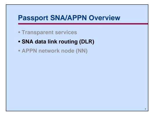
Simply put, the SNA DLR service provides level 2 termination. With this approach, the data link layer is terminated at the point of entry. Data is converted to qualified logical link control (QLLC) for transport across the network and is subsequently converted back to the same or different external media. This service will carry SNA and APPN traffic. The initial version of the service is very similar to the DPN-100 token ring SNA service.
