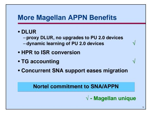
With the Magellan solution, the PU 2.0 devices can be located virtually anywhere in the network and need not be upgraded as the Passport NN acts as a proxy DLUR for the remote PU 2.0 devices.
