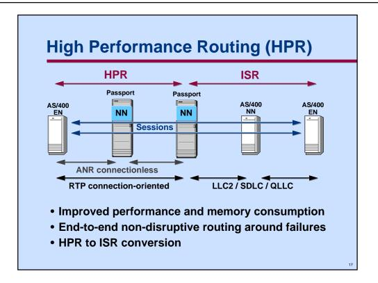
The figure illustrates the protocol stack used by HPR. It includes reliable transport protocol (RTP) which is connection-oriented and provides the reliability. It also includes automatic network routing (ANR) which provides the information required for intermediate nodes to switch data. With HPR, intermediate nodes are not session-aware as opposed to intermediate session routing (ISR) where sessions are terminated and restarted at every APPN node along the path.
