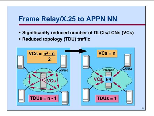
For smaller-scale networks that use the services of a frame relay or X.25 service provider such as is the case with AS/400 or OS/2 networks, introduction of an APPN NN in the network as a value added service can provide significant savings to the end-customer.
