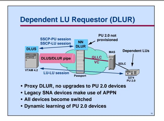
The dependent logical unit requestor (DLUR) operating in conjunction with the dependent logical unit server (DLUS) is designed to alleviate some of the restrictions on dependent LUs. DLUS is only found in a PU type 5 node. It is currently available with VTAM V4R2. One or more DLURs can reside in NNs or ENs.
