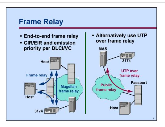
Frame relay has become a very popular way to connect SNA devices as frame relay is natively supported with most IBM devices. Typically, most devices can be made to support frame relay through simple software upgrades.
