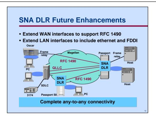
SNA encapsulation over frame relay using request for comments (RFC) 1490 is an upcoming enhancement. This will allow communications with Oscar, frame relay access devices (FRADs), routers, and SNA devices that connect directly to frame relay.
