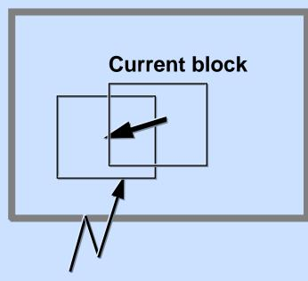
Previously stored YUV numbers for the most similar old block, which are the estimate for the current block's YUV
