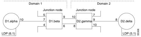
The **dspnwrt** command must be entered at node D1.alpha or D2.delta (the end points of the connection).
