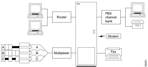
A circuit line is the physical line that carries frame relay, data, voice, or ATM traffic between customer equipment and an IPX or IGX node. Each piece of equipment in the illustration above is attached to the node through a circuit line. After a card has been "upped" with the upcd command, a circuit line on that card can be "upped" and configured.
