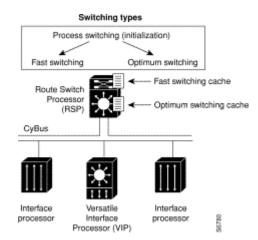
The VIP card installed in this router maintains a copy of the routing cache information needed to forward packets. Because the VIP card has the routing information it needs, it performs the switching locally, making the packet forwarding much faster. Router throughput is increased linearly based on the number of VIP cards installed in the router.
