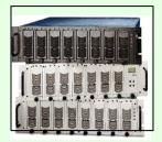
An acronym for Redundant Array of Independent Disks, a family of techniques for managing multiple disks to deliver desirable cost, data availability, and performance characteristics to host environments.
