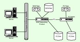
The SoIP Framework is an open, standards-based architecture for deploying native IP storage solutions using the IP Storage standards within the IETF IP Storage Working Group such as iSCSI and iFCP.
