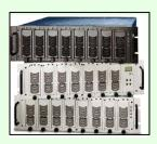
Acronym for "Just a Bunch Of Disks." Originally used to mean a collection of disks without the coordinated control provided by control software; today the term JBOD most often refers to a cabinet of disks whether or not RAID functionality is present.
