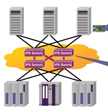
Use the existing Fibre Channel adapters, RAID controllers, and storage management software
