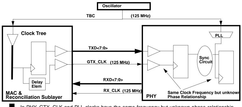
In PHY, GTX\_CLK and PLL clocks have the same frequency but unknown phase relationship. Need to account for the synchronization delay in PHY in the Bit Budget calculation.
