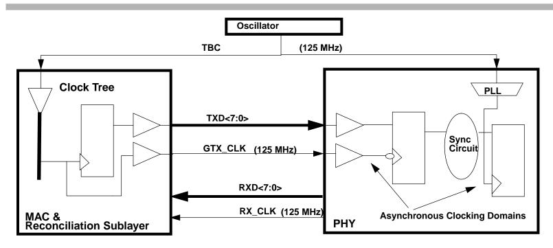
**Data Clocking:** Launch at Rising clock edge & latch at the falling clock edge.
