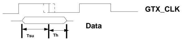
The duty cycle for GTX\_CLK needs to within 40 to 60% and its rise and fall times should be bounded as in Gigabit-10b interface to be from 0.7 to 2.4ns.
