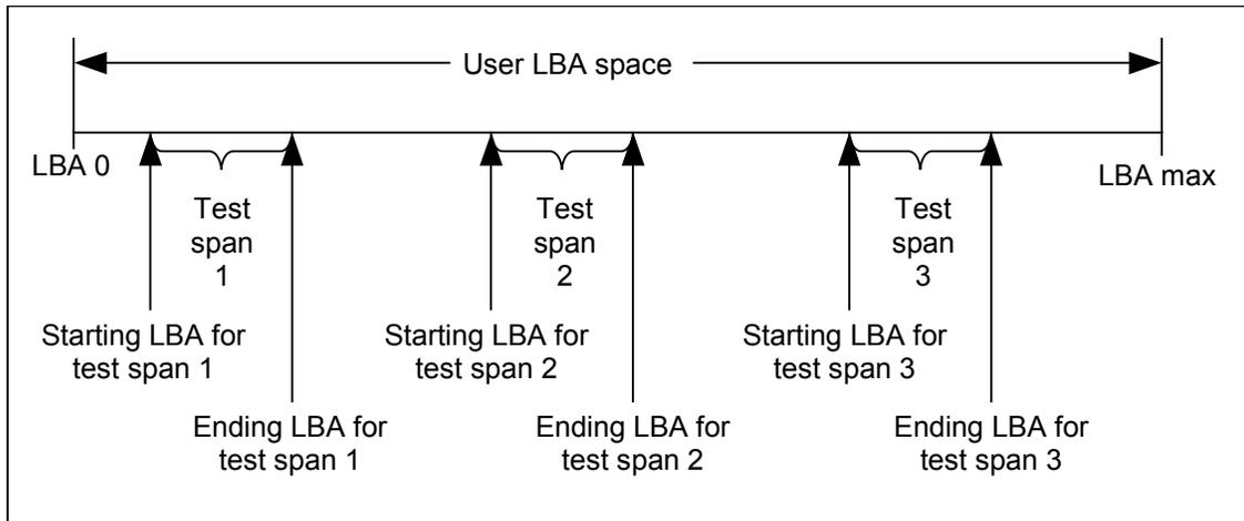
**Figure 7 – Selective self-test test span example**
