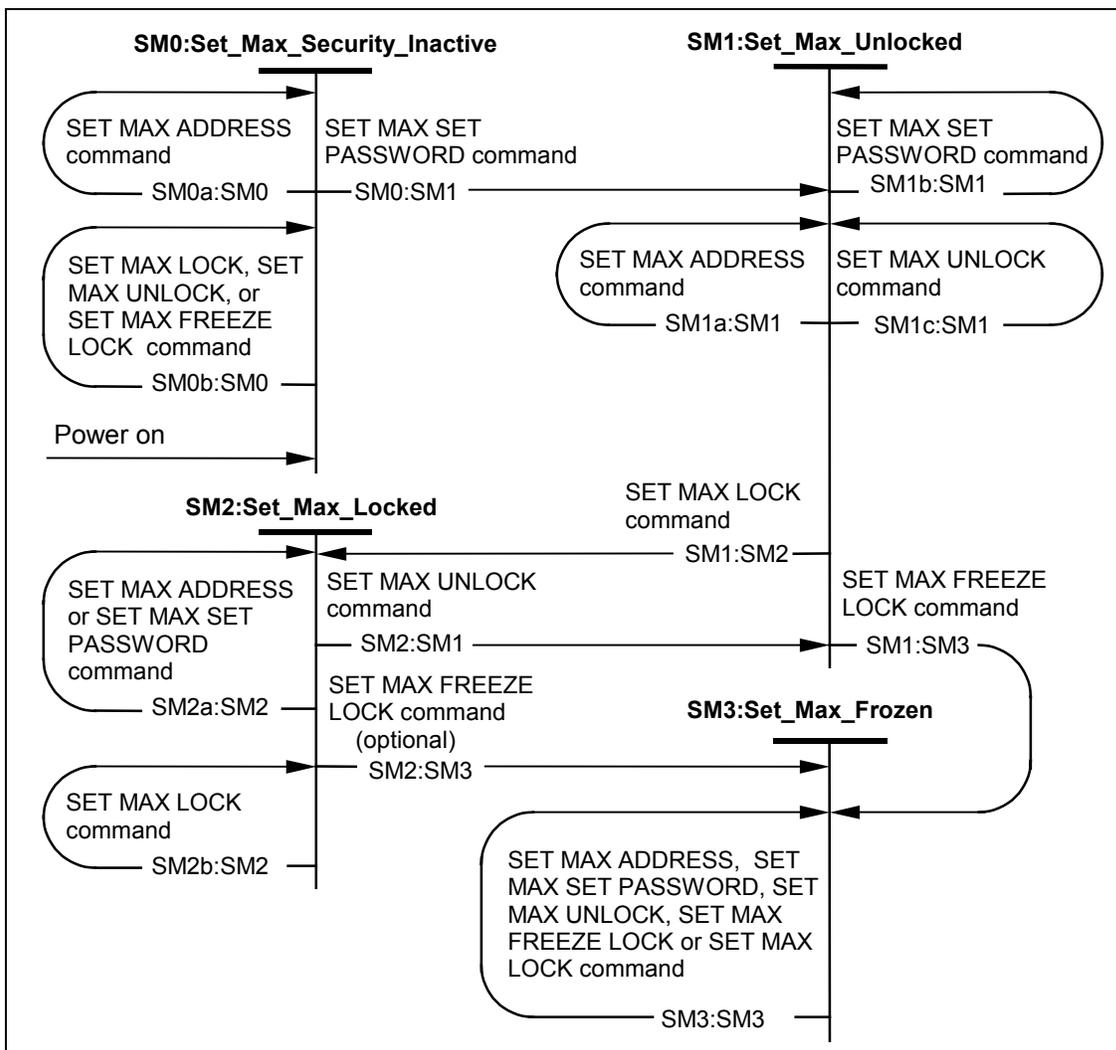
Figure 5 – SET MAX security state diagram
