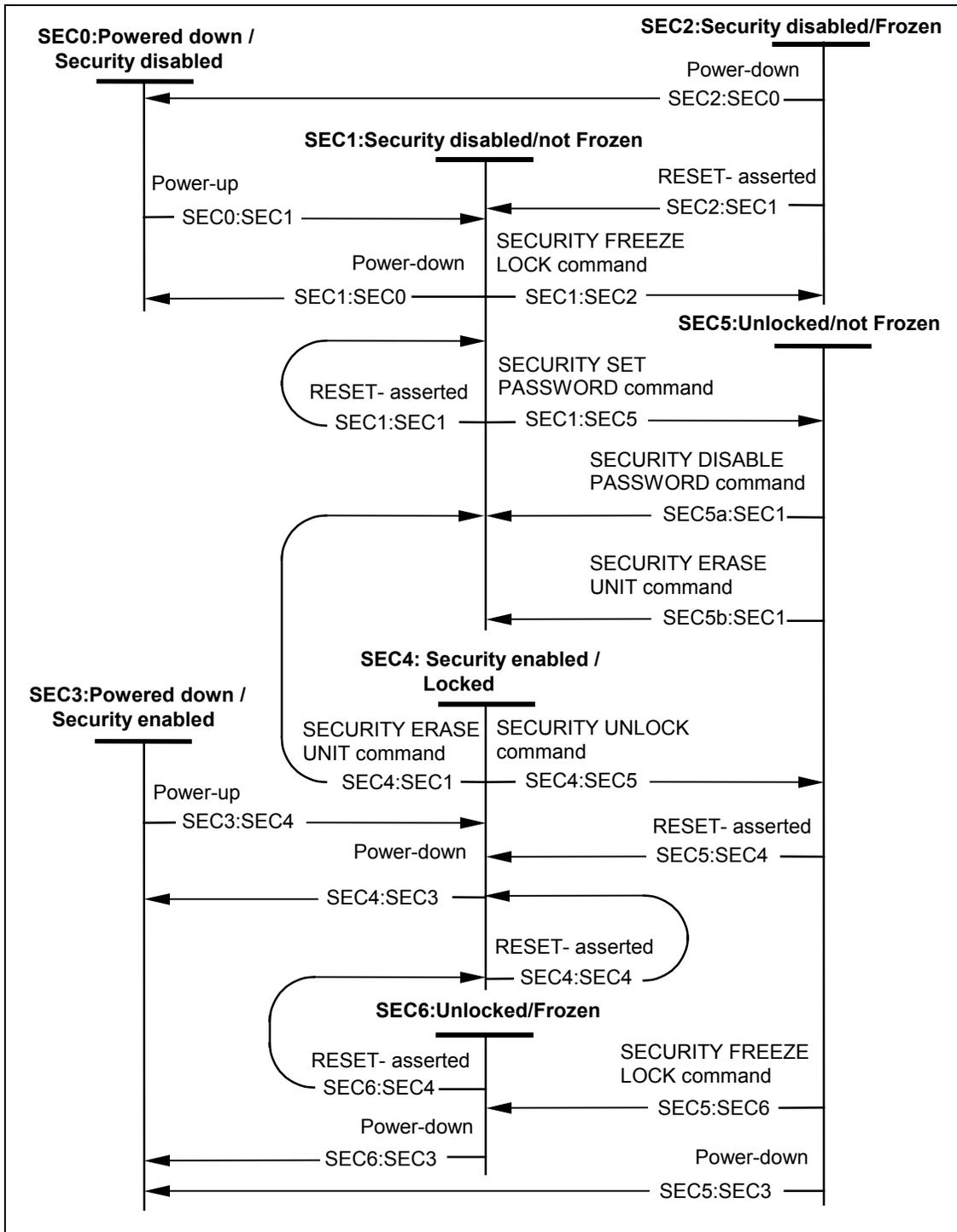
Figure 4 – Security mode state diagram
