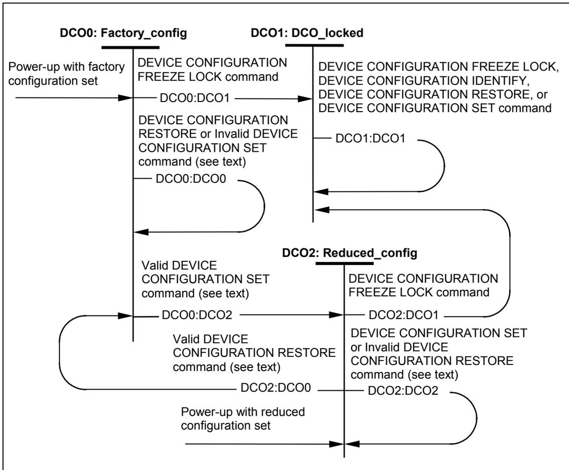
Figure 6 – Device Configuration Overlay state diagram
