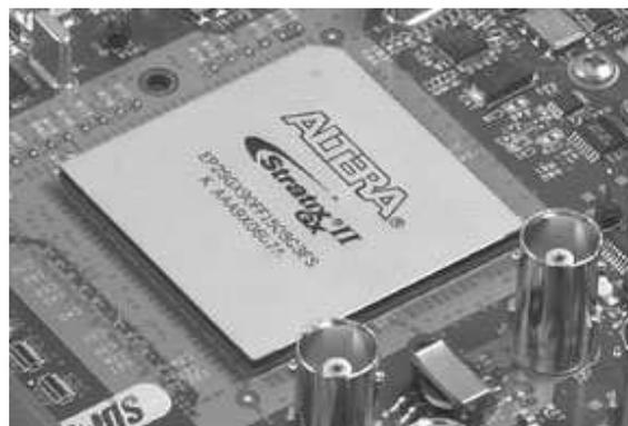
*3.3.1 An Altera Stratix II GX FPGA*
