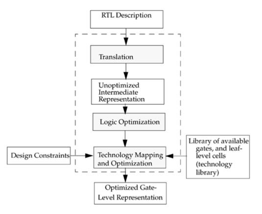
Figure 14-4. Logic Synthesis Flow from RTL to Gates
