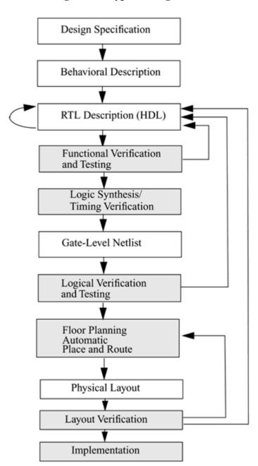
Figure 1-1. Typical Design Flow
