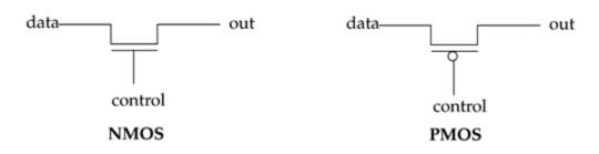
Figure 11-1. NMOS and PMOS Switches
