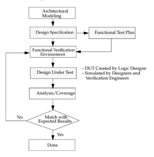
Figure 15-1. Traditional Verification Flow
