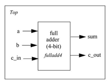
Figure 4-3. I/O Ports for Top and Full Adder
