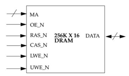
Figure F-2. DRAM Input/Output Ports
