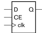
FIGURE 4.5 A D flip-flop with clock-enable input.
