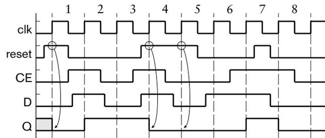
FIGURE 4.8 Timing diagram for a flip-flop with clock-enable and synchronous reset inputs.
