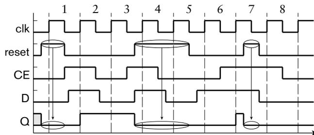
FIGURE 4.9 Timing diagram for a flip-flop with clock-enable and asynchronous reset inputs.
