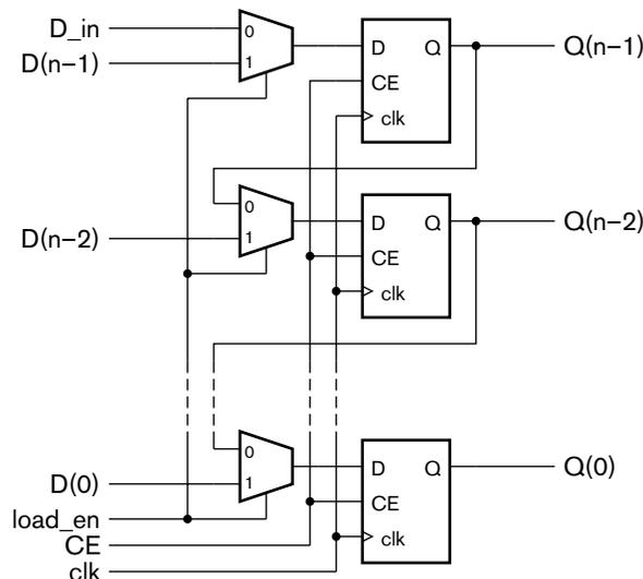
FIGURE 4.12 A shift register implemented with D flip-flops and multiplexers.
