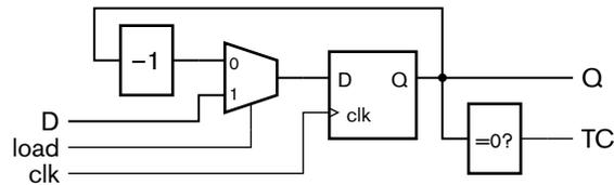
If the clock input to the counter is a periodic signal with period  $t$  and the counter is loaded with a value  $k$ , the terminal count is reached after an interval of  $k \times t$ . Thus, this form of counter can be used as an *interval timer*, where the terminal-count output signal is used to trigger an activity after expiration of a given time interval.
