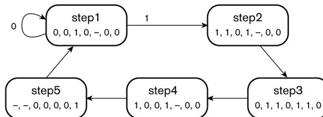
FIGURE 4.34 State transition diagram for the complex multiplier.
