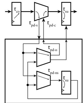
FIGURE 4.38 Control path in a digital system.
