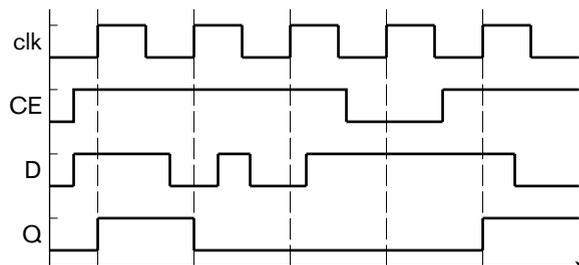
FIGURE 4.6 Timing diagram for a D flip-flop with clock enable.
