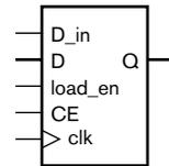
FIGURE 4.11 A symbol for a shift register.
