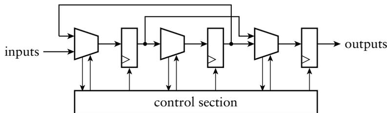
FIGURE 4.35 A general view of a digital system.
