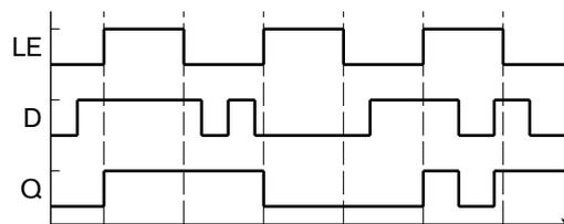
FIGURE 4.15 Timing diagram for a latch.
