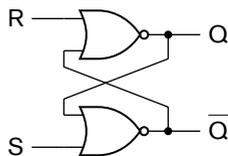
FIGURE 4.18 Cross-coupled RS-latch.
