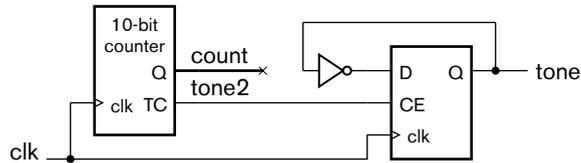
FIGURE 4.25 Timing diagram for an alarm clock frequency divider.
