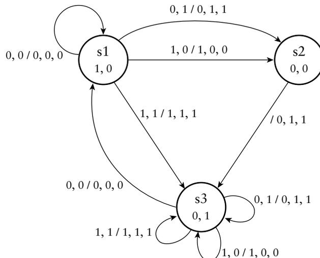
FIGURE 4.33 A state transition diagram augmented with Moore- and Mealy-style output values.
