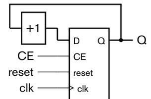
FIGURE 4.22 A counter with clock-enable and reset inputs.
