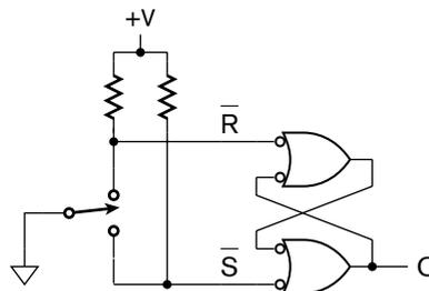
FIGURE 4.45 A switch debouncer using an RS-latch.
