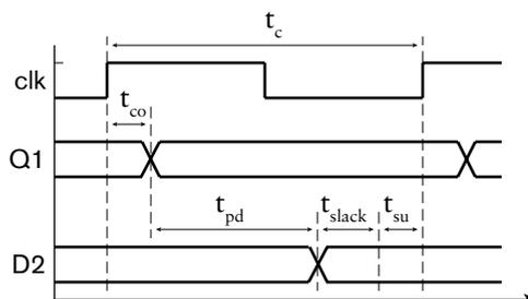
FIGURE 4.37 Register-to-register timing.
