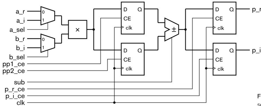
FIGURE 4.30 Datapath for a sequential complex multiplier.
