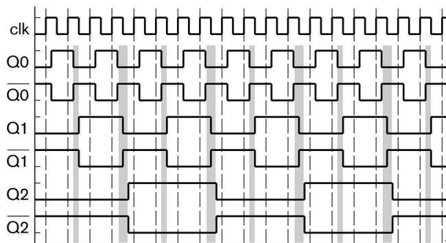
flip-flop) changes from 1 to 0. In general, we can think of the flip-flops for bits 0 to  $i - 1$  as forming an  $i$ -bit counter. The most significant bit of this counter changes from 1 to 0 when it overflows. When that happens, the next flip-flop, for bit  $i$ , toggles between 0 and 1. This behavior is shown in the timing diagram of Figure 4.29.
