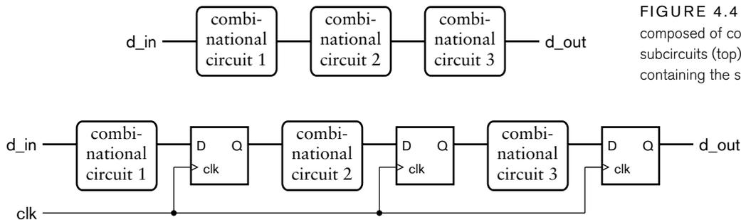
FIGURE 4.4 A circuit composed of combinational subcircuits (top), and a pipeline containing the same subcircuits.
