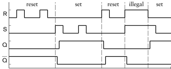
FIGURE 4.19 Timing for an RS-latch, showing the reset and set states, as well as an illegal operating condition.
