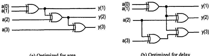
Figure 6.19 Delay constraint implementation.
