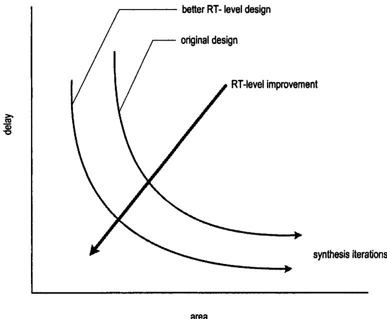
**Figure 6.20** Synthesis iterations and the impact of RT-level change.
