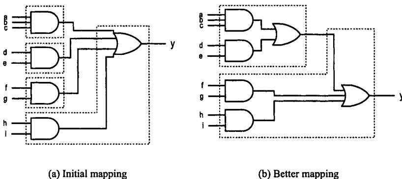
**Figure 6.11** LUT-based FPGA technology mapping example.
