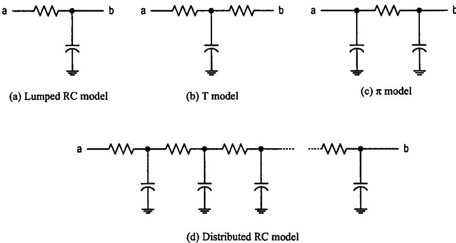
**Figure 6.15** Wiring models.
