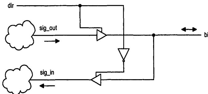
Figure 6.4 Dual-buffer bidirectional I/O port.
