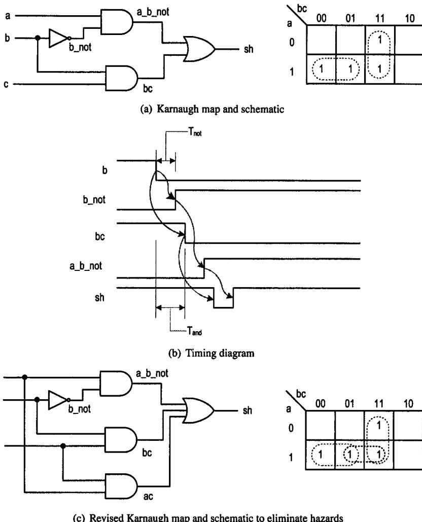
Figure 6.21 Static hazards example.
