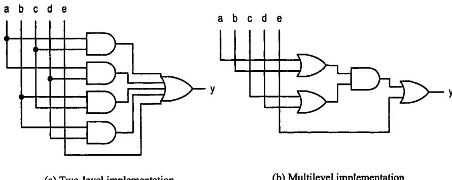
**Figure 6.8** Two-level versus multilevel implementation
