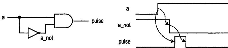
Figure 6.23 Delay-sensitive edge detection circuit.
