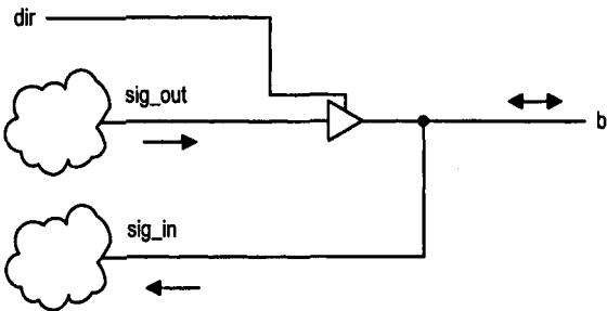
Figure 6.3 Single-buffer bidirectional I/O port.
