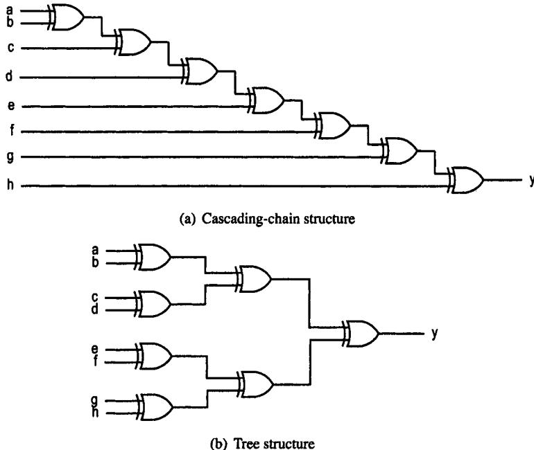
**Figure 6.13** Routing structures of an odd-parity circuit.
