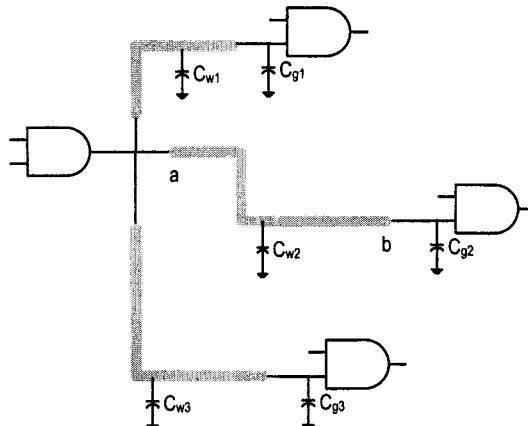
**Figure 6.14** Delay estimation at the cell level.
