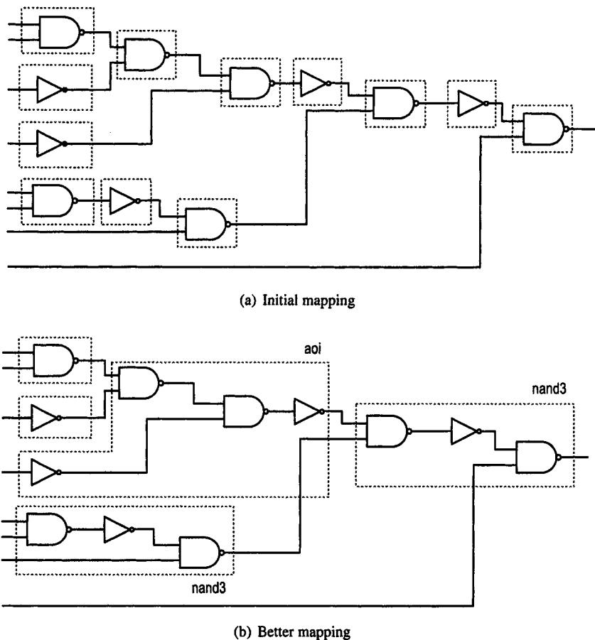
**Figure 6.10** Standard-cell technology mapping example.
