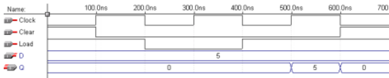
Figure 8.3. Sample simulation trace for the 4-bit register.
