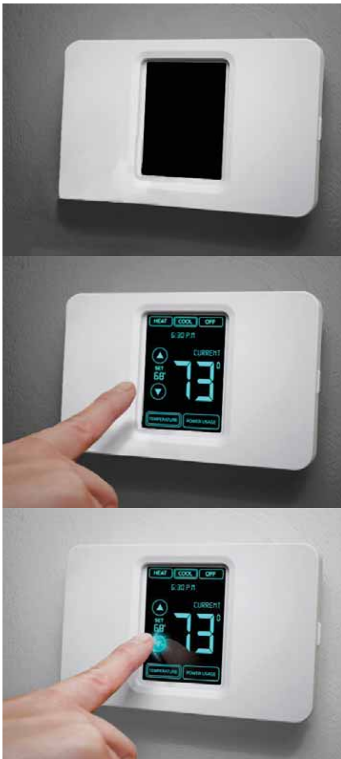
An animation of a hand approaching a dead-fronted thermostat and it waking-up.
