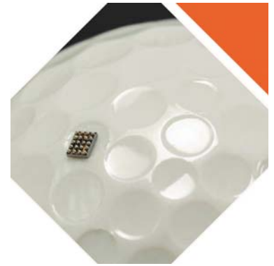
Figure 2: The NXP Kinetis KL03 20-pin ARM® Cortex®-M0 powered MCU, at 1.6 mm x 2.0 mm, is suitable for ingestible healthcare sensing. The KL03 (MKL03Z32xxx4) supports 32 KB Flash, 2 KB SRAM, 8 KB boot ROM, and up to 22 GPIO.
