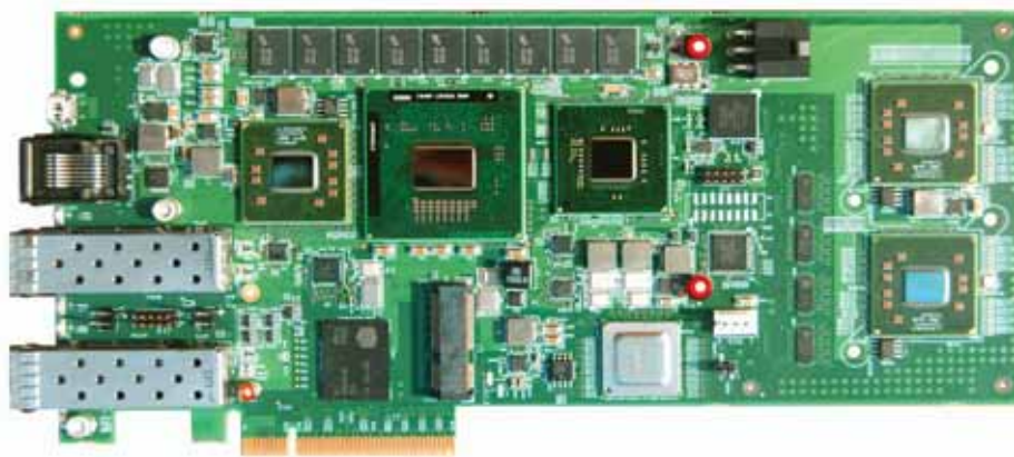
Figure 3. The WIN SoNIC (IP-90380), an instantiation of the Next Generation Communications Platform from Intel®.
