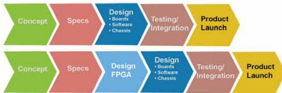
Figure 1. An FPGA approach essentially adds a separate fork of development cycle for the FPGA circuit (which can be viewed as a product in and of itself).
