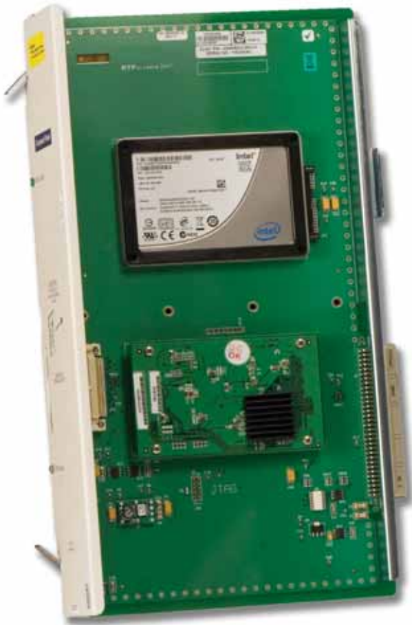
Figure 2. Removable drives must be compatible with hardware at the data offload point.
