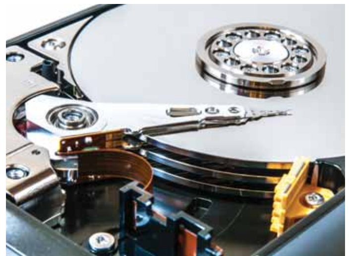
Figure 2. Inside a mechanical disk drive. (Image courtesy of William Warby; http://bit.ly/1iaFTed .)
