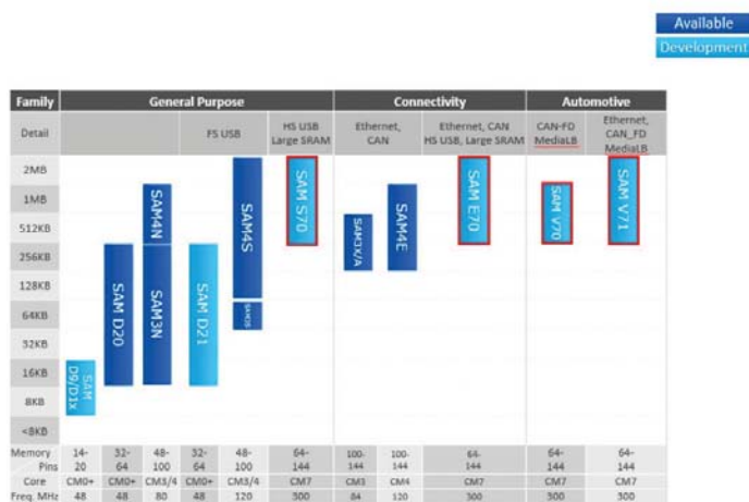
Figure 1: The Cortex-M7 based, general-purpose SAM S70, the connectivity-focused SAM E70, and the automotive-qualified SAM V70 and SAM V71 add to the existing SAM MCU family from Atmel.
