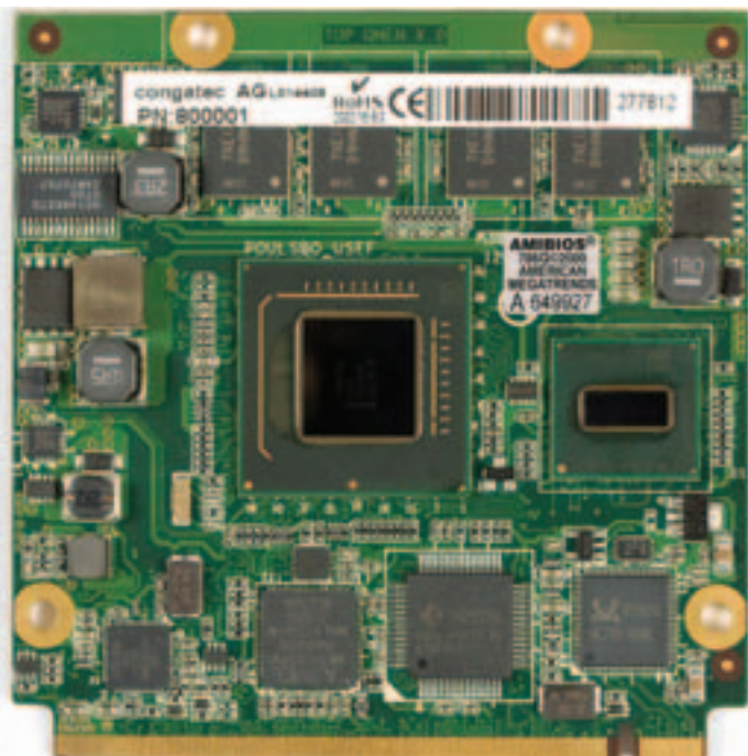
Figure 2: This top view shows a congatec Qseven design.
