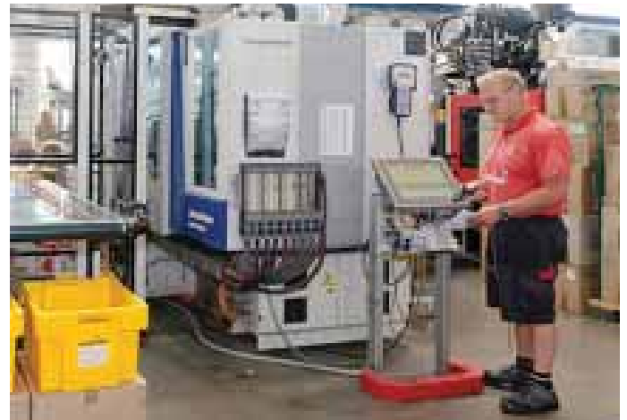
Figure 1. Rugged, sealed panel PC used in manufacturing.
