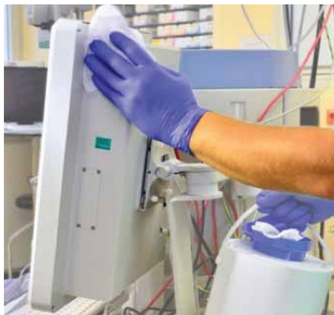
Figure 3. Close-up of wipe-down disinfecting process. No moisture will penetrate the IP65 interior.
