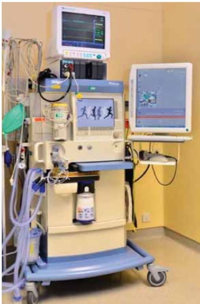
Figure 2. Cart-mounted medical PC is fully sealed and able to withstand disinfectants and “substantial” liquids.
