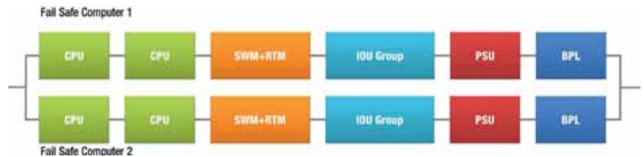
Figure 3. The implementation of a dual 2oo2 architecture to deliver high availability.
