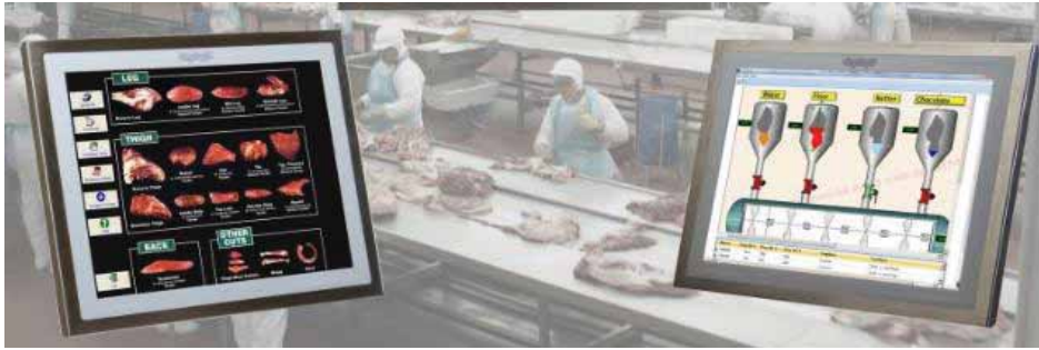
Figure 4. Examples of food processing PCs, also fully sealed and supporting high-temp liquid washdown.
