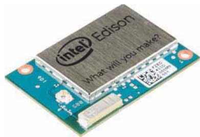
Figure 1: The Intel Edison mini-computer is now slightly larger than an SD card, but with increased I/O, more software support, and higher computing performance as compared to the original, launched at CES 2014.
