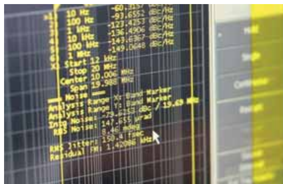
Figure 6: The total jitter of the notional system shown in Figure 5 using Pericom demo boards in the same bench set-up as Figure 4. Total additive jitter is a mere 0.15 ps (RMS).
