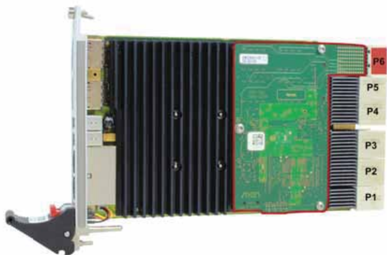
Figure 2: This mezzanine features a P6 backplane connector for Ethernet configuration of the system slot CPU.
