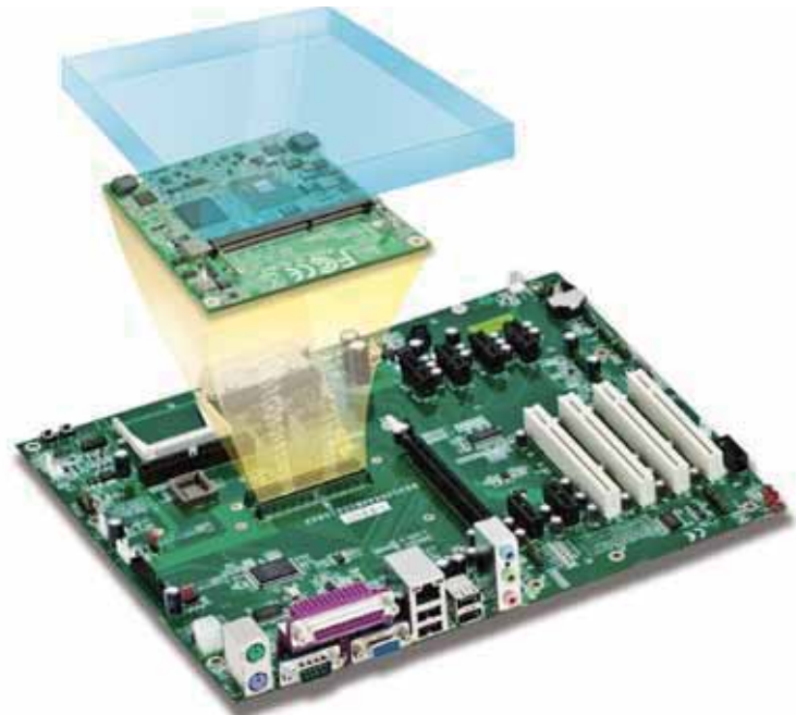
Figure 1: COM Express modular architecture enables upgradability, flexibility, expandability and faster time to market.
