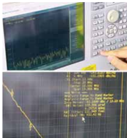
Figure 4: Using a phase noise analyzer by Agilent (top) and a LeCroy 6 GHz scope (bottom), the jitter of the demo board from Figure 3 is shown to be 0.111 ps (shown as 111.949 fs).
