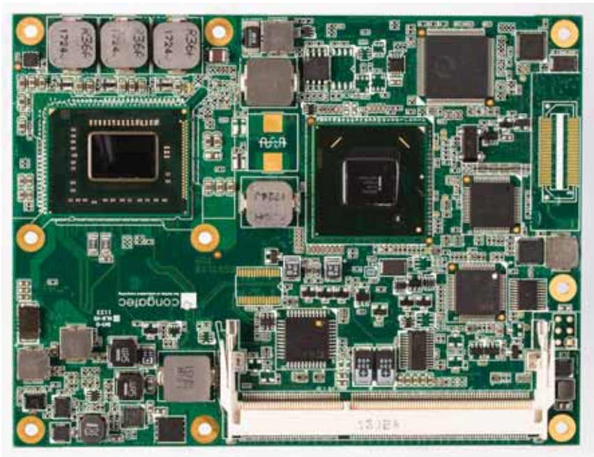
Figure 3: The computing core of the ZES Zimmer's power analyzer: congatec's conga-BS77 COM Express module with 3rd generation Intel® Core™ i5 processor
