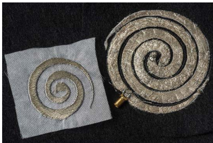
Figure 3: Ohio State University is working on integrating antennas and circuits into clothing for the future of healthcare monitoring and treatment. (Source: Ohio State University)
