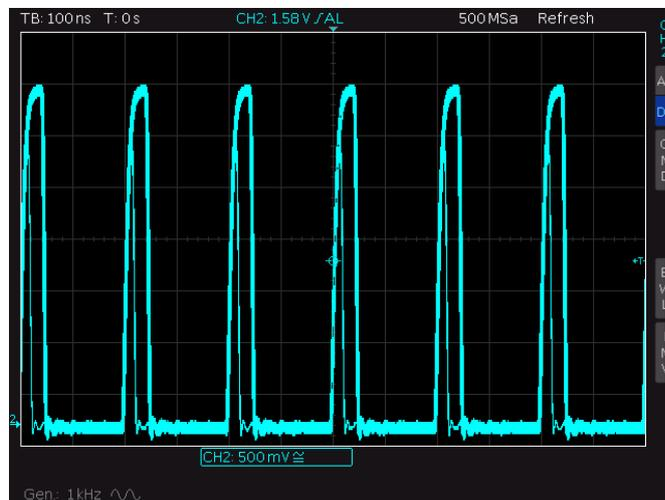
Fig. 33: Pulse packet with a glitch.
