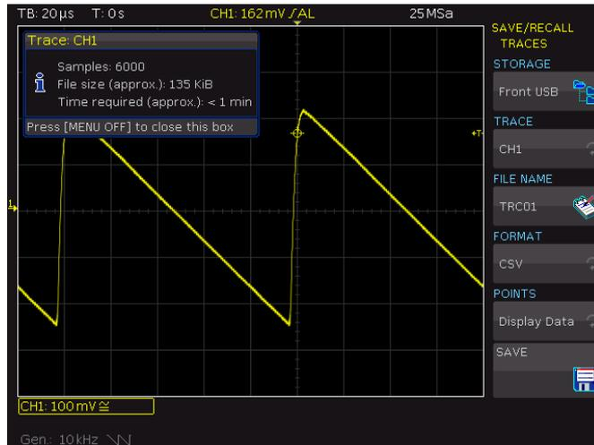
Fig. 27: Saving an acquired signal.
