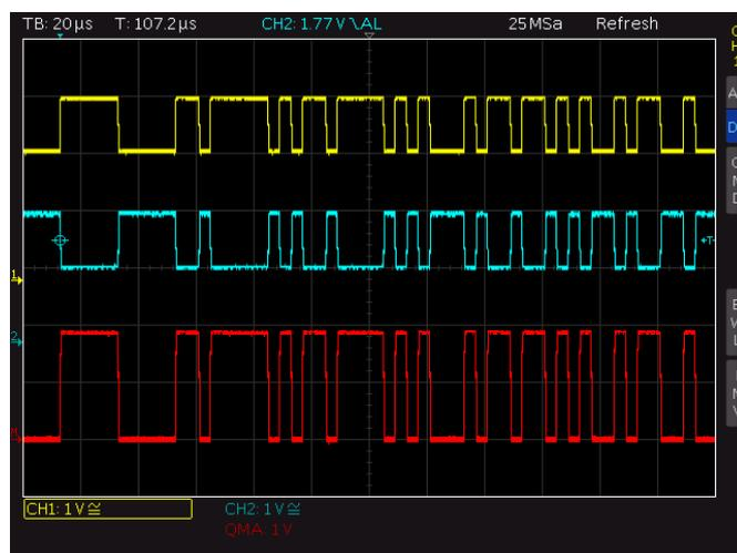
Fig. 44: Measuring differential signals.
