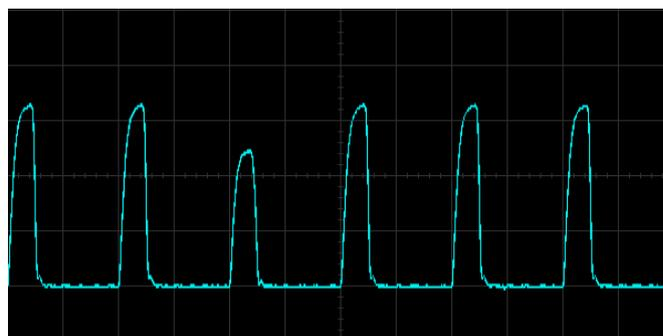
Fig. 35: Triggering a runt pulse.
