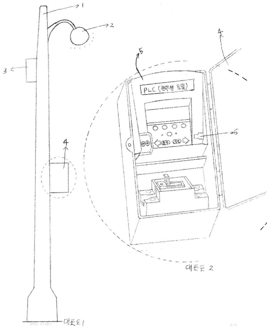
. PLC(Power Line Communication). Carrier - current transceiver
