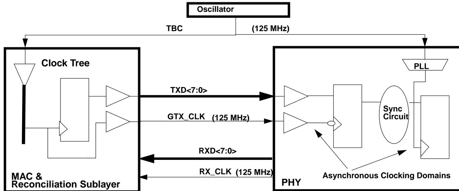
**Data Clocking:** Launch at Rising clock edge & latch at the falling clock edge.
