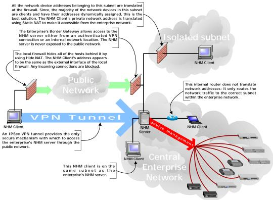
Another Horizon Manager client in Figure 7 is in an isolated subnet outside of the central enterprise network, but within the enterprise. This subnet contains dynamically assigned RFC 1918 addresses for all the desktop workstations within the subnet. To prevent address collisions
