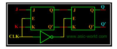
In the figure above there are two latches, the first latch on the left is called master latch and the one on the right is called slave latch. Master latch is positively clocked and slave latch is negatively clocked.
