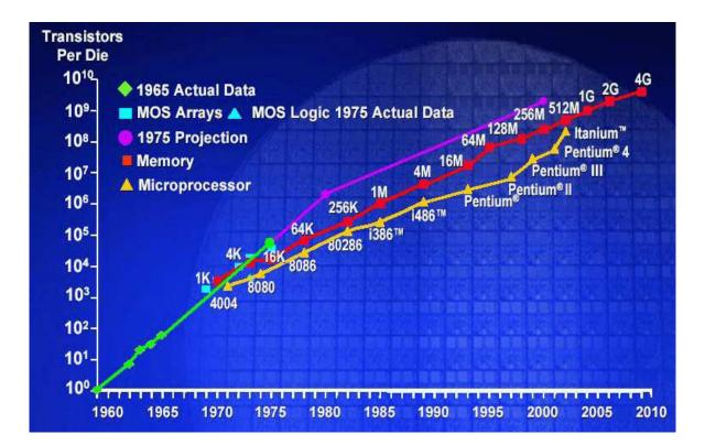
The growth of complexity of integrated circuits follows a trend called "Moore's Law", first observed by Gordon Moore of Intel. Moore's Law in its modern interpretation states that the number of transistors in an integrated circuit doubles every two years. By the year 2000 the largest integrated circuits contained hundreds of millions of transistors. It is difficult to say whether the trend will continue.
