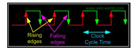
A clock signal is a periodic square wave that indefinitely switches from 0 to 1 and from 1 to 0 at fixed intervals. Clock cycle time or clock period: the time interval between two consecutive rising or falling edges of the clock.
