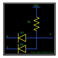
If X = 0 and Y = 0, then both diodes D1 and D2 are forward biased and thus both diodes conduct and pull F low.
