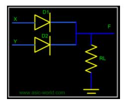
If X = 0 and Y = 0, then both diodes D1 and D2 are reverse biased and thus both the diodes are in cut-off and thus F is low.
