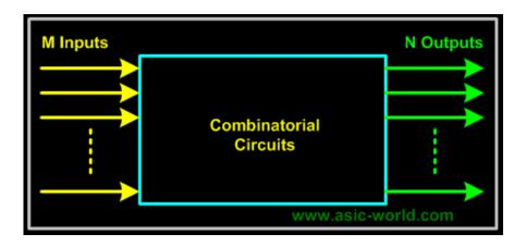
Whenever the same set of inputs is fed in to a combinatorial circuit, the same outputs will be generated. Such circuits are said to be stateless. Some simple combinational logic elements that we have seen in previous sections are "Gates".
