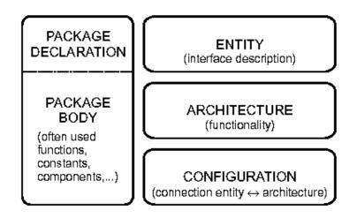
In VHDL one generally distinguishes between the external view of a module and its internal description. The external view is reflected in the entity declaration, which represents an interface description of a 'black box'. The important part of this interface description consists of signals over which the individual modules communicate with each other.
