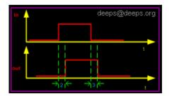
Normally we can have three models of delays, typical, minimum and maximum delay. During compilation of a modules one needs to specify the delay models to use, else Simulator will use the typical model.
