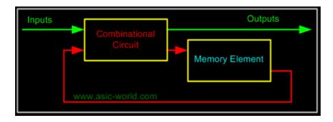
The memory elements are devices capable of storing binary info. The binary info stored in the memory elements at any given time defines the state of the sequential circuit. The input and the present state of the memory element determine the output. Memory elements next state is also a function of external inputs and present state. A sequential circuit is specified by a time sequence of inputs, outputs, and internal states.
