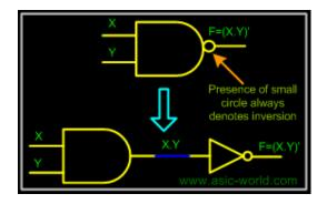
If X and Y are two inputs, then output F can be represented mathematically as F = (X.Y)', Here dot (.) denotes the AND operation and (') denotes inversion. Truth table and symbol of the N AND gate is shown in the figure below.
