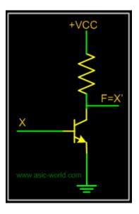
When X = 1, the transistor input pin 1 is HIGH, this produces the forward bias across the emitter base junction and so the transistor conducts. As the collector current flows, the voltage drop across RL increases and hence F is LOW.
