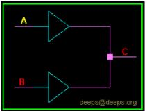
Two buffers that has output A : Pull 1 B : Supply 0 Since supply 0 is stronger then pull 1, Output C takes value of B.
