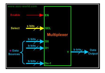
MUX acts like a digitally controlled multi-position switch where the binary code applied to the select inputs controls the input source that will be switched on to the output as shown in the figure below. At any given point of time only one input gets selected and is connected to output, based on the select input signal.
