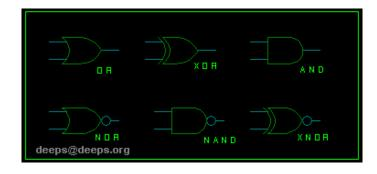
The gates have one scalar output and multiple scalar inputs. The 1st terminal in the list of gate terminals is an output and the other terminals are inputs.
