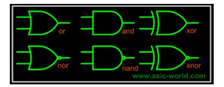
All the gates in the above figure have 2 inputs and one output; combinational elements simplest form are "not" gate and "buffer" as shown in the figure below. They have only one input and one output.
