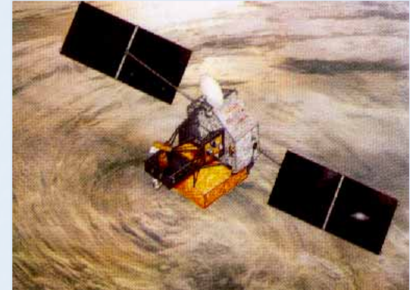
Tropical Rainfall Measuring Mission (TRMM) satellite equipped with world first rain radar developed by NICT/JAXA
