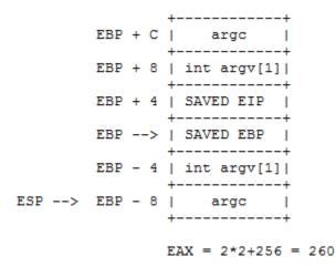
Now it's time to return to main(). Knowing that sub's return value of 260 in in EAX, it wipes down its stack frame in line <+27> by adding 8 to ESP. Then it pops the value in ESP(after adding 8 to ESP) which is the SAVED EBP into EBP register. Then it uses the SAVED EIP to return to main() (line <+60>).
