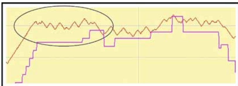
Dedicated in-vehicle devices that employ high-frequency sampling provide accurate observations of a driver's behaviour. They can identify bad behaviour such as tailgating (Figure 2a left) – see how brown line shows excessive speed changes; and detect details like gear changes (Figure 2b right). This type of detailed information is particularly useful when accidents need to be reconstructed. Purple shows data from GPS data at 1 sample per second and Brown is high-frequency sampling of speed sensor data - Graphics courtesy Redtail Telematics.
