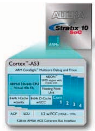
Figure 4: Stratix 10 contains four Cortex-A53 cores, ARM's most impressive multi-threaded 64-bit core.
