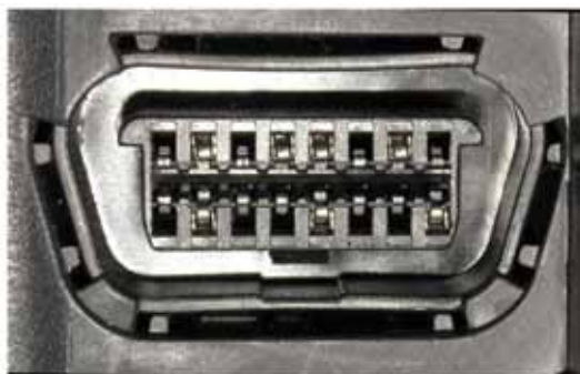
Figure 1a (left): Typical OBD-II Port is easily accessible under the car dashboard. Figure 1b (right): Danlaw's DataLogger 7-Series is a small, self-installed, OBD connected telematics solution.
