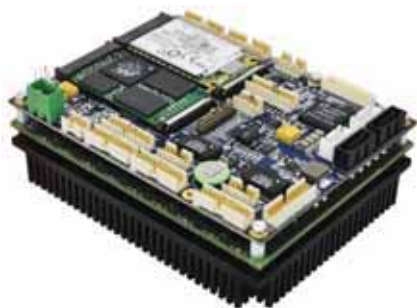
Figure 2: Connect Tech's CCG011COM Express® Type 6 Rugged Ultra Lite Carrier Board uses locking, rugged pin headers and supports extended temperature ranges of -40°C to +85°C.
