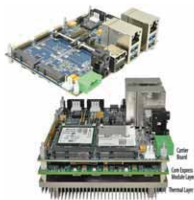
Figure 1: Connect Tech's CCG008 COM Express® Type 6 Ultra Lite Carrier Board uses standard PC-style connectors for interfaces such as USB, Ethernet, serial and video.
