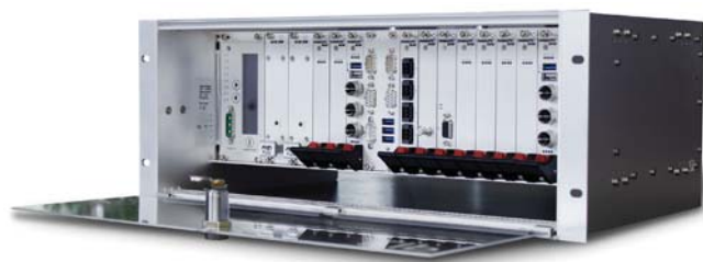
Figure 2: CompactPCI Serial enables high-performance train IT platforms in a compact 19-inch 4U form factor with fanless operation and EN 50155 qualification.
