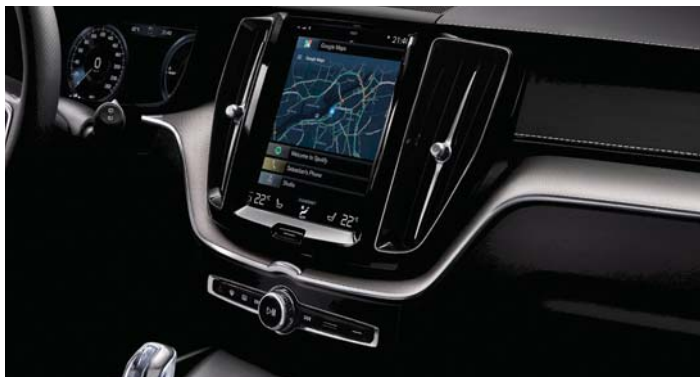
Figure 1: Proposed Google Volvo XC60 interior. Volvo announced plans to use a Google Android-based infotainment and connectivity solution that is fully integrated beyond traditional smartphone-based IVI, extending to the instrument cluster, HVAC control, window/mirror/seat adjustment, and other IVI, in-cab functions. (Image: Volvo)
