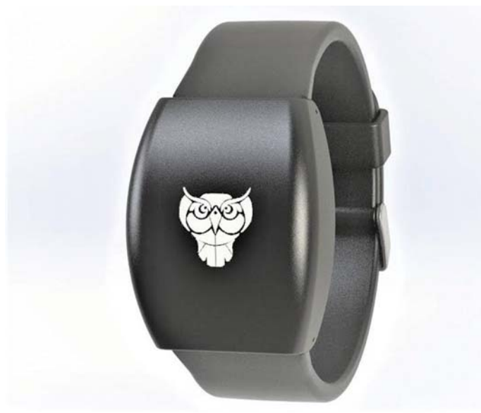
Figure 3: A biometric sensor capable of discovering drowsiness so as to avert its becoming hazardous.
