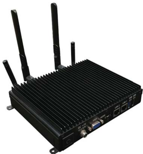
Figure 3: IoT-380 Gateway with Intel® Atom™ Processor E3800 SoC. (Image source: WIN Enterprises)
