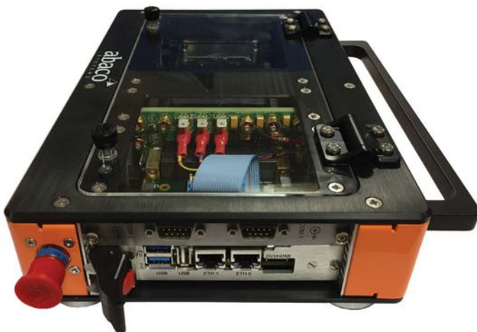
Figure 2: A conduction-cooled SBC314 (choice of T2081/T1042 PowerPC processor) 3U VPX single board computer
