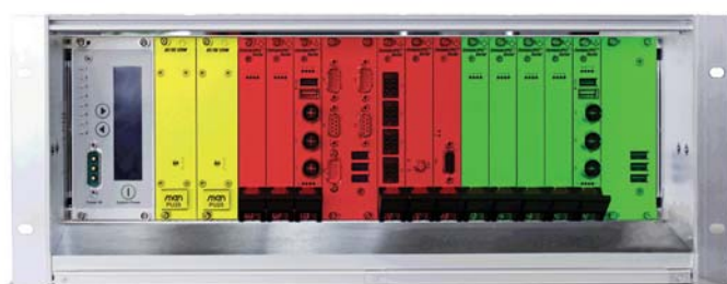
Figure 3: Two in one: Two cards—connected over the backplane via Ethernet—and a redundant power supply in a single system.
