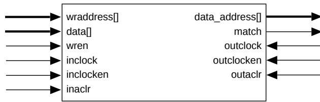
Figure 23. APEX 20KE CAM Block Diagram
