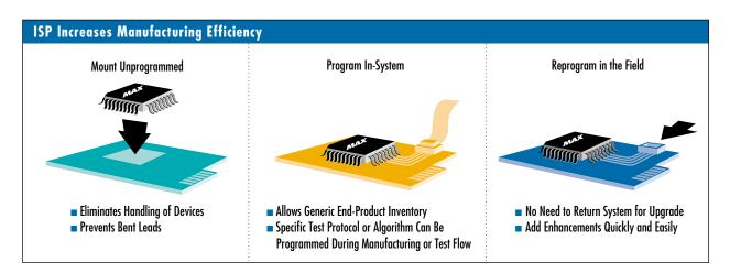
MAX 7000A, MAX 7000S, MAX 7000B, MAX 3000A, and MAX 9000 devices provide an industry-standard four-pin JTAG ISP interface for programming a device after it has been mounted on a printed circuit board.
