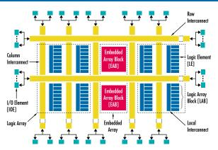
The FLEX 10K family is the first programmable logic device family with an embedded array.
