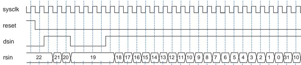
**Figure 5. Using *dsout* to Control Output of Data from the Decoder**
