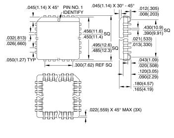
**28LW**, 28-pad, Windowed, Ceramic Leadless Chip Carrier (LCC)
