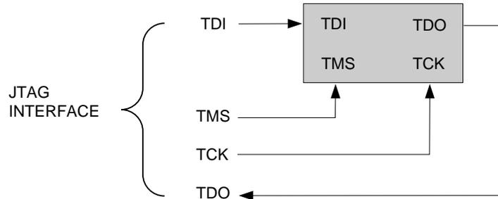
**Note:** You will need to reserve space on your circuit board to accommodate a 10-pin male header for the JTAG interface. The pinout for this header must match the Atmel ISP
