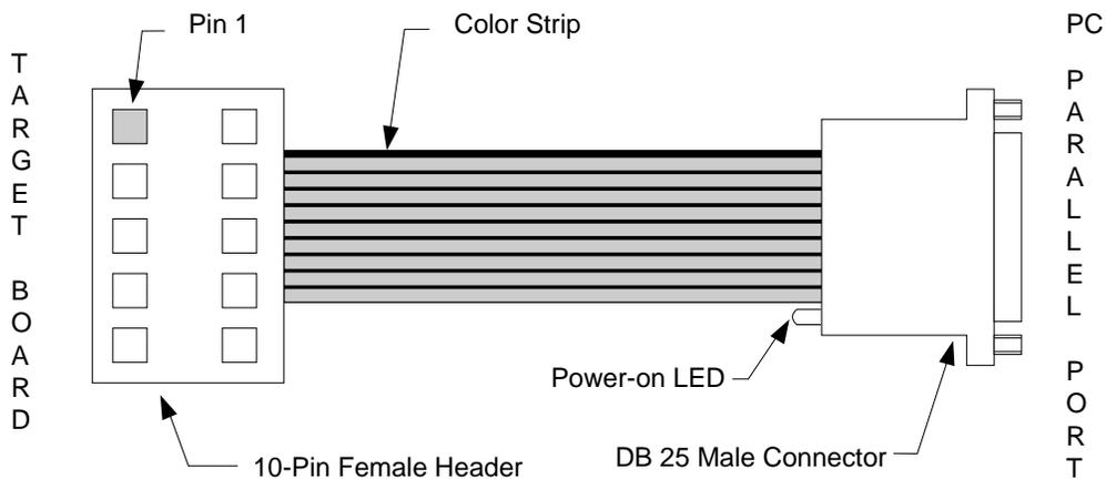
Figure 5 shows the pinout for the 10-pin Female header on the Atmel ISP cable. The pinout on the 10-pin Male Header on your circuit board *must* match this pinout.
