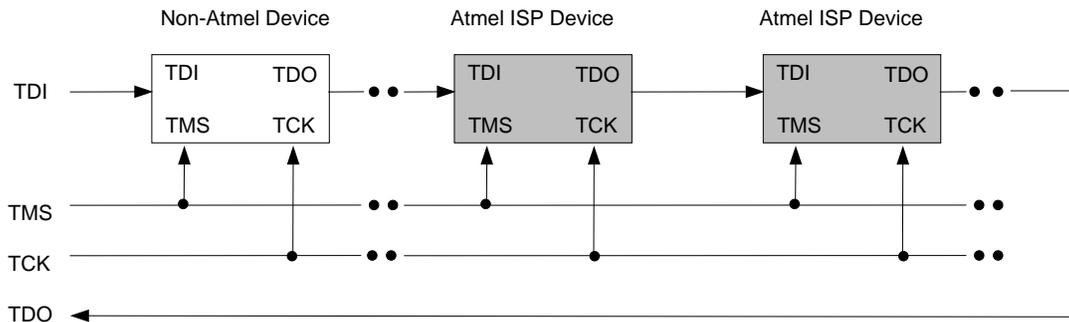
TDI, TMS, TCK and TDO comprise the JTAG interface. The ISP software allows you to create a JTAG daisy chain for multiple devices, including non-Atmel devices, and implement Parallel ISP for Atmel devices.
