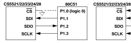
Figure 1. 3-Wire and 4-Wire Interfaces
