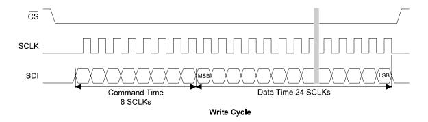
Figure 4. Write-Cycle Timing
