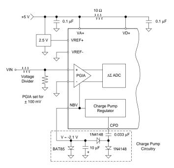
Figure 1. CS552X ADC with Charge Pump
