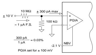
Figure 2. Resistor Divider for  $\pm 10$  V Input
