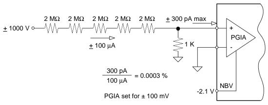
Figure 4. Resistive Divider for Very High Voltage
