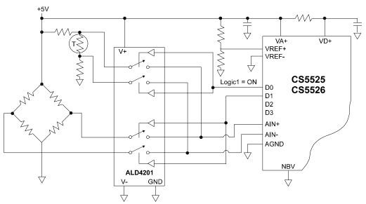
Figure 5. CS5525/CS5526 Controls the low-voltage ALD4201 analog switch.
