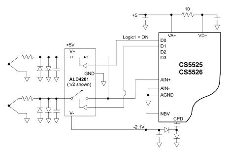
Figure 4. CS5525/CS5526 Controls the low-voltage ALD4201 analog switch.
