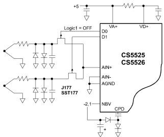
Figure 2. CS5525/CS5526 Controls P-Channel JFETs as analog switches.
