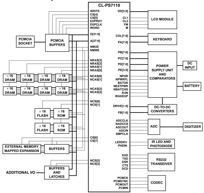
A separate synchronous serial interface supports two industry-standard protocols (SPI® and Microwire®) for interfacing to standard devices such as an ADC, allowing for peripheral expansion such as the use of a digitizer pen.
