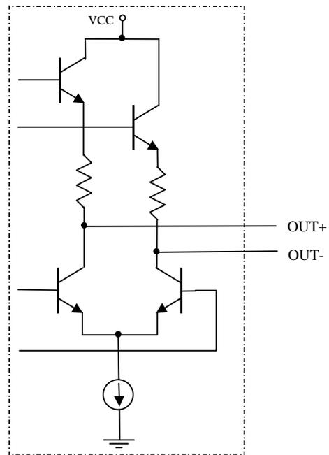
Figure 6. LVDS output structure
