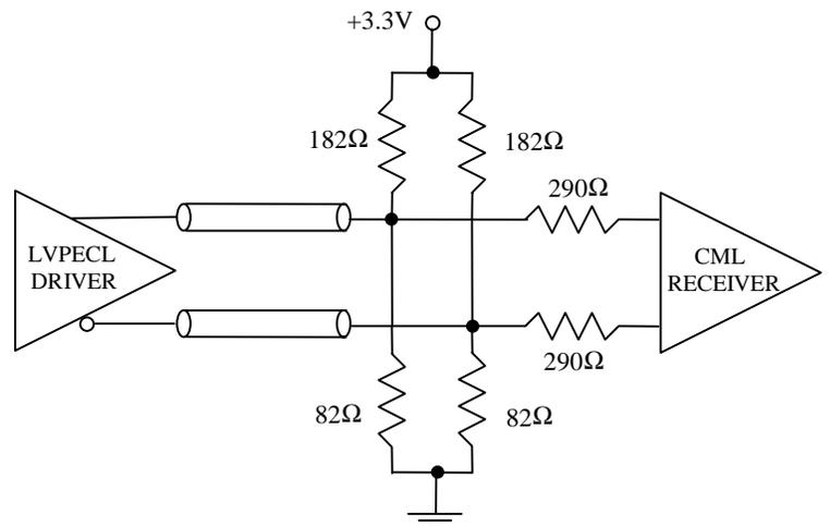
Figure 15. DC-coupling between LVPECL and CML (MAX3875)
