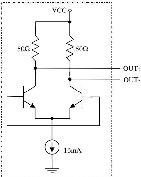
Figure 3. CML output structure
