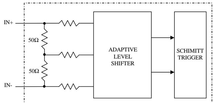
Figure 7. LVDS input structure
