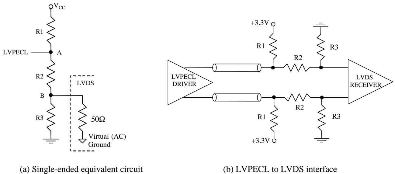
Figure 17. DC-coupling between LVPECL and LVDS
