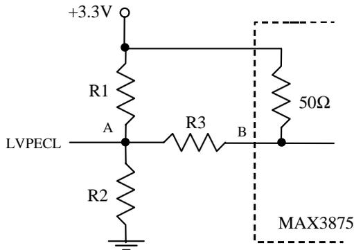
Figure 14. Resistor network between LVPECL and CML (MAX3875)
