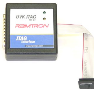
Figure 10: Versa-JTAG interface for programming and debugging the VRS51L2070
