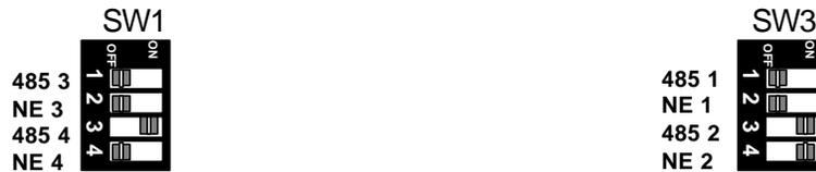
Figure 2: RS422/485 Interface Configuration
